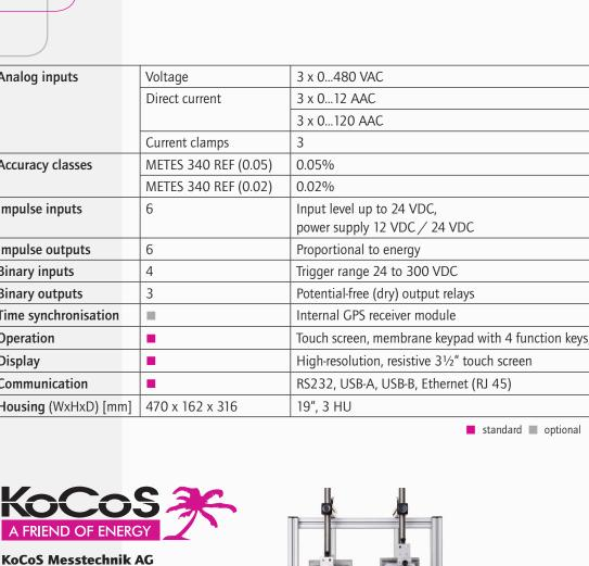
In METES 340 REF an active USB interface has been integrated for data transfer via USB storage media, while an Ethernet interface allows direct integration in any network.
